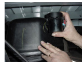
Step 3: Slide fuel valve from bracket.
