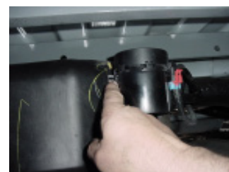
Step 2: Disengage the locking pin.
